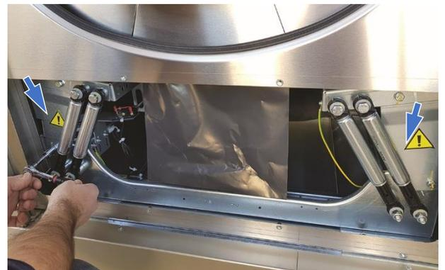
Then remove the 2 clamps at the rear of the washing machines by removing the protective panel of each washing machine, using a 30 mm Torx key.
