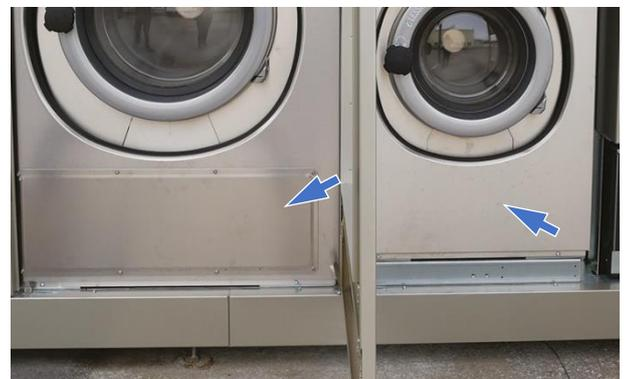
Remove the 2 transport clamps on the front of the washing machines with a 10 mm socket spanner (8 kg) and a 13 mm socket spanner (20 kg).
